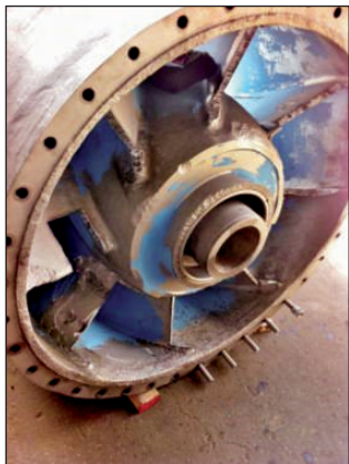
The severely eroded vanes were cut away.
